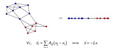
Eigenvectors of  $L \rightarrow$  eigenmodes Eigenvalues of  $L \rightarrow$  levels of energy
