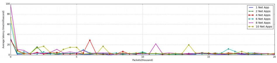
Processing time for delivering 20 thousands packet\_in messages to 1-10 network applications
